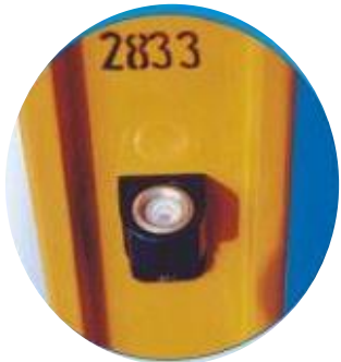
Has a circular bubble, Metal base Prevent corrosion of staff base
