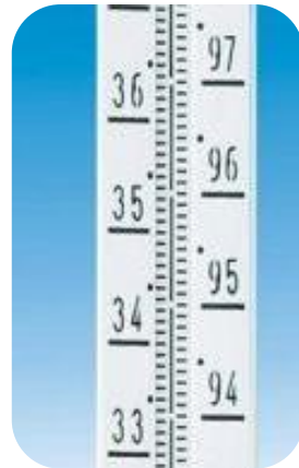
More accurate Sometimes min. division 0.5cm (double that of ordinary staff)
